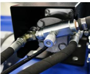
Clamping chuck is powered by a **variable speed hydraulic motor**, including low speed valve for tyre tread sculpting : 1.5, 2, 3 ... 9 rpm.
