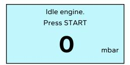
Start the vehicle engine and keep it idling. Press ENTER START to start the particulate filter check
