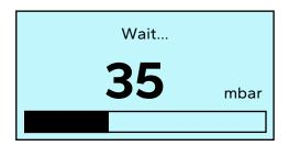
During this phase the measurement is performed and the instantaneous pressure in mbar is displayed. After a few seconds the message with the measurement result appears
