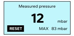
Start the vehicle engine to take the measurement. The instantaneous pressure is displayed in the center of the screen, while the maximum pressure detected during the measurement session is displayed in the lower right corner.
