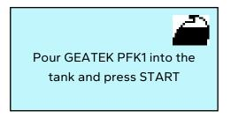
Press ENTER START to inject GEATEK PFK1 into the particulate filter
