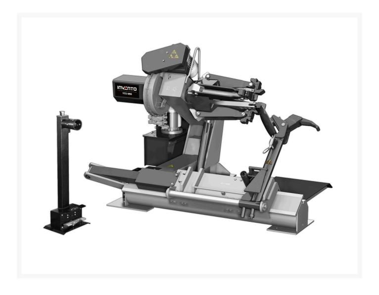
**INVENTO TCS 656** tyre changer is an economic machine used to service wheels of lorries, agricultural and construction vehicles. The machine has a manually raised arm and a rotating disc. The ergonomic and portable control panel ensures convenient work from either side of the machine. Dual speed nut speeds up the operation.
