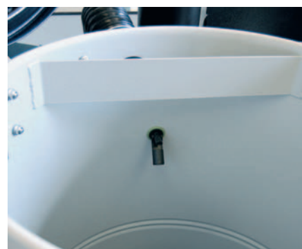
AUTOMATIC LEVEL CONTROL
