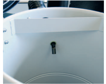
AUTOMATIC LEVEL CONTROL
