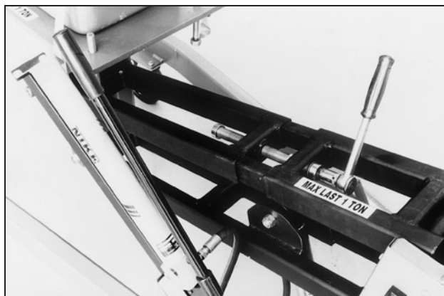
Stepless tipping of the fixing device plate length-wise by catch.
