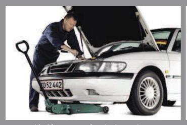
Ideal for support of engine/transmission components during repair, with vehicle in low height.
