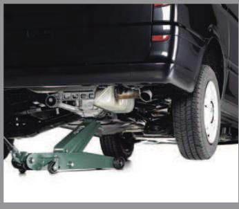
Low chassis height improves access to lifting points deep under most vehicles.
